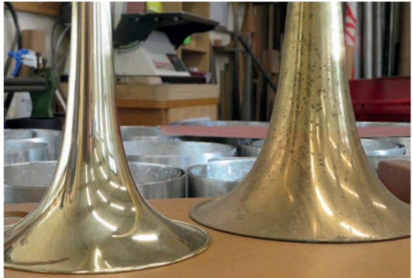
▲ Orchestral trumpet resonators: before cleaning (right), and after (left)
