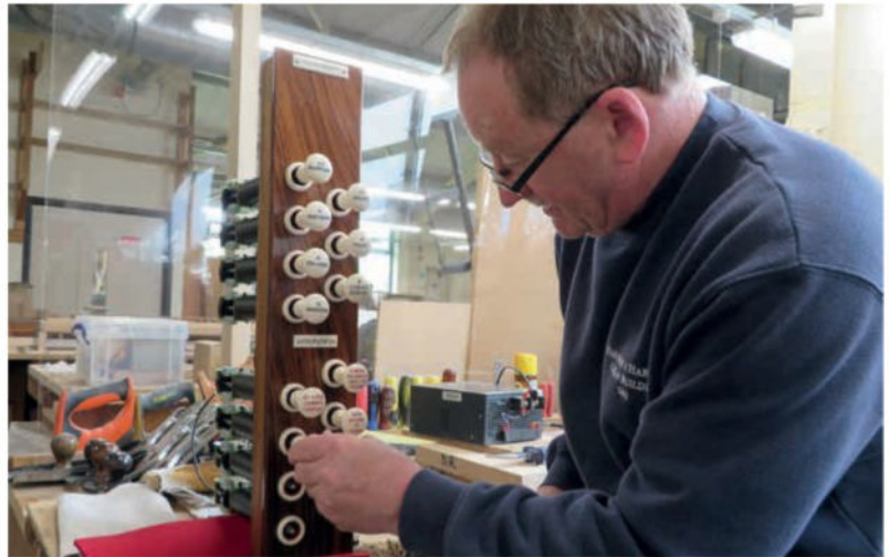
▼ David Robinson tests the electro-pneumatic action of the stop jams
