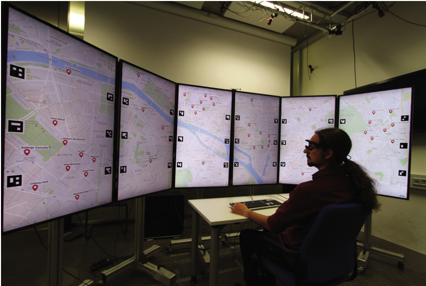
Figure 2.25 Showing a geographic map on a large-scale display while the observer is equipped with an eye tracking device for either exploring where he is paying visual attention or for using the eye tracker as gaze-assisted interaction (figure provided by Lars Lischke).
